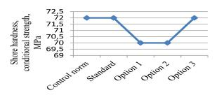
Fig. 4. Shore hardness of vulcanizates
