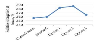
Fig. 3. Relative elongation of vulcanizates during elongation
