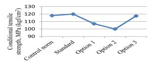
Fig. 2. Conditional tensile strength of vulcanizates
